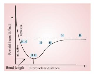
Fig. 7.9 Potential energy diagram for formation of a hydrogen molecule
