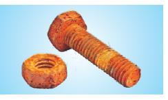
Fig. 4.9: Rusted nuts and bolts of iron
