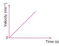
Fig. 9.24 velocity-time graph of an object moving with uniform acceleration
