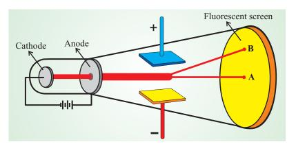
**Fig. 5.2:** The cathode rays are negatively charged; these travel in straight line from cathode to the anode (A), however in the presence of an external electrical field these bend towards the positive plate (B)
