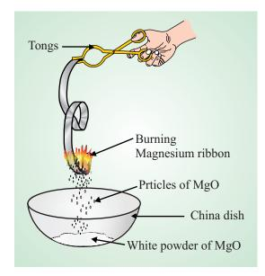
Fig. 4.1: Burning of magnesium ribbon
