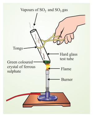
Fig. 4.3: Thermal decomposition of ferrous sulphate
