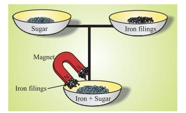
Fig. 2.15 : Magnetic Separation of a mixture
