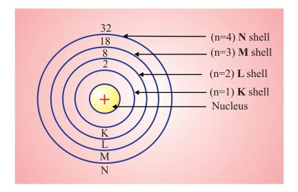
Fig. 5.8: Illustration showing different orbits or the energy levels of fixed energy in an atom according to Bohr's model
