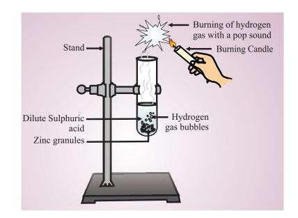
**Fig. 8.1:** Experiment to study the reaction of dil.  $H_2SO_4$  with zinc. The gas burns with a 'pop' sound when a burning match stick is brought near the mouth of the test tube.
