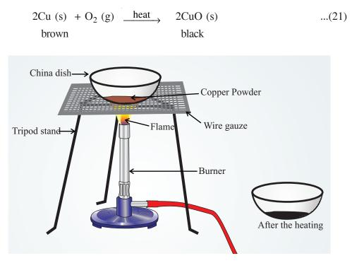
Fig. 4.7: Heating of copper powder in air
