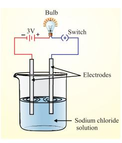
Fig. 7.7 Aqueous solution of sodium chloride conducts electricity
