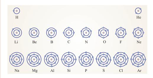
Fig. 5.10: The structures, according to Bohr's model of atoms, of elements with atomic number 1 to 18.
