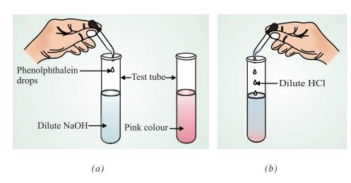
Fig. 8.4: Reaction between NaOH and HCl (a) Pink colour solution containing NaOH solution and a drop of phenolphthalein (b) The solution becomes colourless on addition of dil HCl
