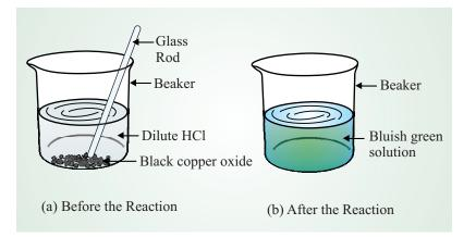
**Fig. 8.3** Reaction between dilute hydrochloric acid and copper oxide (a) before reaction black particles of copper oxide in transparent dilute hydrochloric acid and (b) after reaction bluish green solution.
