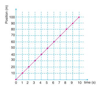
Fig. 9.20 Position-time graph for the motion of a particle on the basis of data given in table
