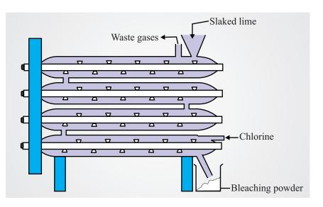
Fig. 8.10 Hasen-Clever plant for manufacturing of bleaching powder
